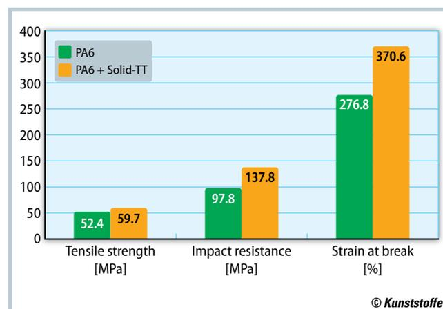
**Fig. 2.** Testing of the mechanical properties of PA6 (Nycoa 1637) with Solid-TT in comparison with unfilled, processed polymer revealed increased strain at break and impact resistance
